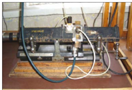
This instrument for measuring electrical field distribution in microwave waveguides was originally developed more than 70 years ago, but is still in good working condition in one of the teaching labs at KhNURE.
