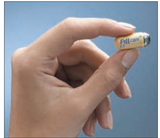
Given Imaging Pill-cam, the smallest camera (you can swallow it) made in Israel. Courtesy of Given Imaging.
